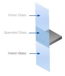
Spandrel glass or "non-vision glass" are used on several buildings to conceal essential components that no one wants to see and are typically located below or on top of the vision glass on each floor of the building.
